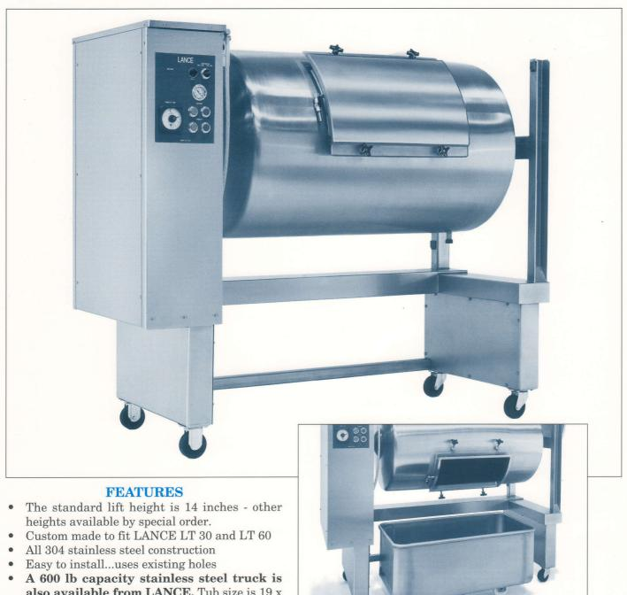
• A 600 lb capacity stainless steel truck is also available from LANCE. Tub size is 19 x 31 x 45 inches. Overall height is 27 inches. Constructed in the USA of 304 stainless steel. Shown in use with LANCE LT 60 with 14 inch LANCE LIFT KIT installed.
