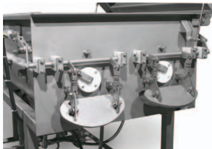
Air operated discharge doors (discharge cover must be in place when unit is in operation)
