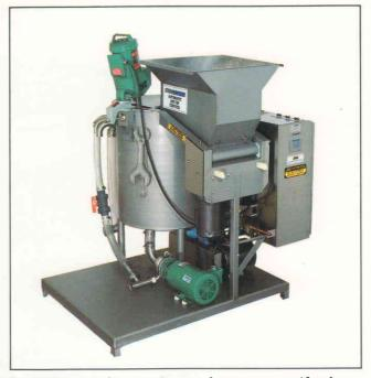
The batter transfer pump system features a centrifugal pump with special batter blender impeller. Thorough blending is assured because the impeller breaks up any lumps in the dry mix. A by-pass valve controls the amount of mixed batter that can be recirculated within the ABC-II. The mixer is designed for connection to an inplant water supply.
