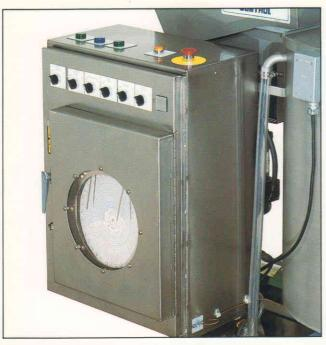
Stein's control system provides continuous viscosity monitoring and control. Control box is water tight for reliability.
