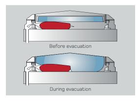
**Expansion Cushion** with **Snap-out Frame** reduces evacuation time by up to 30% and prevents wrinkles on the upper side of the package.
