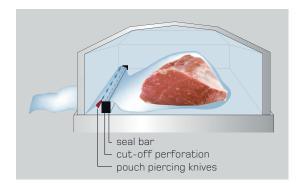
Pouch Piercing Knives (optional) pierce evacuation slots into overlength bags which protrude from the chamber so that the closing lid cannot obstruct evacuation. (Not necessary for machines with Trim Removal System).
