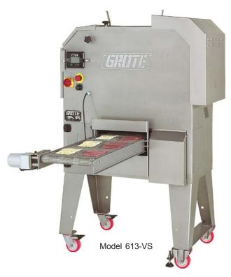
Bulk slices, stacks, and shingles into portions at rates from 37 up to 90 strokes per minute, per lane.
