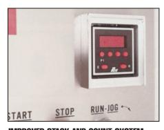
**IMPROVED STACK AND COUNT SYSTEM** The state-of-the-art counter is not limited by the number of patties. You are able to set the counter for any number of patties in a 6" high stack.
