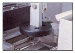
**SIDE NOTCH PAPER INTERLEAVING SYSTEM** Unique design eliminates constant adjusting competitive systems require. The knock out cup assembly does not need adjustment every time K.O. cup is changed, reducing changeover time.
