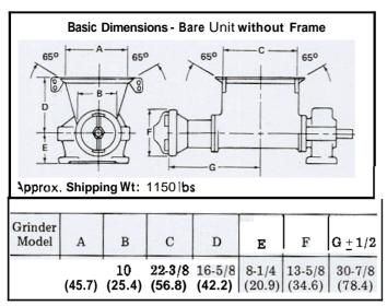
NOTE: Hopper extensions or guards not shown. Height of support legs shown would be determined by desired discharge height. Add leg length to D or E for overall height or discharge clearance.
