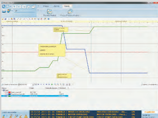
Diagrams of batch temperature, vacuum and drum speed in time-function.
