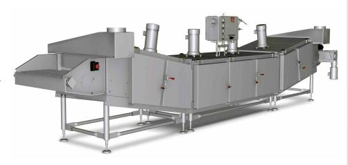
incoming product load and temperature variations. Internal fan system maintains production capacity and helps ensure evenly chilled products. These standard features add to the effective conservation of cryogen and optimize overall freezer performance.
