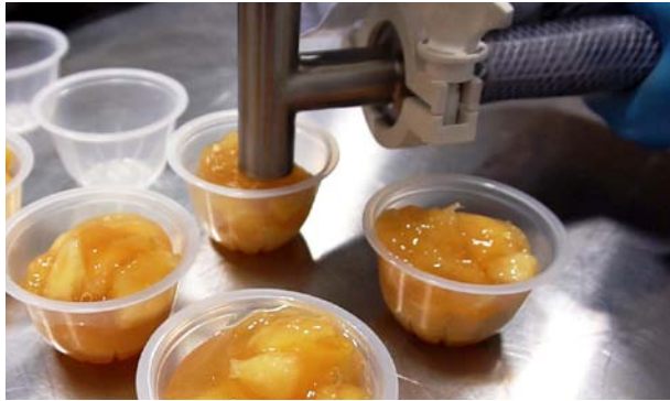
Above: Hand depositing nozzle filling cups with apple pie filling. Below: 1" vertical cut-off spouts filling jars with mustard.
