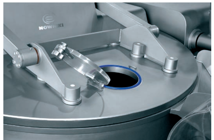
check opening hole abertura de control
