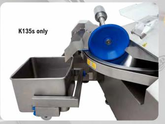
**Hydraulic bin loader** and hydraulic unloader arm with **motorized extracting disc, variable speed** 50-150 rpm.
