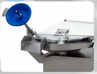
Manual unloader arm with **motorized extracting disc, variable speed** 50-150 rpm.
