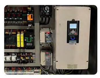
Soft start and stop of knifes, bowl and extracting disc (optional) by mean of speed drives.
