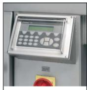
PLC for setting of pump pressure & speed. Constant read-out of current brine temperature.
