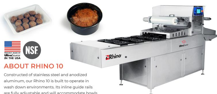
aluminum, our Rhino 10 is built to operate in wash down environments. Its inline guide rails are fully adjustable and will accommodate bowls, trays, cups, and more. The wide sealing area accommodates three rows of #3 size trays that are advanced by a stepper motor into the sealing mold, sealed, and then automatically discharged. Tooling changeover is fast and easy, requiring a single tool to accomplish product changeovers in less than 15 minutes.
