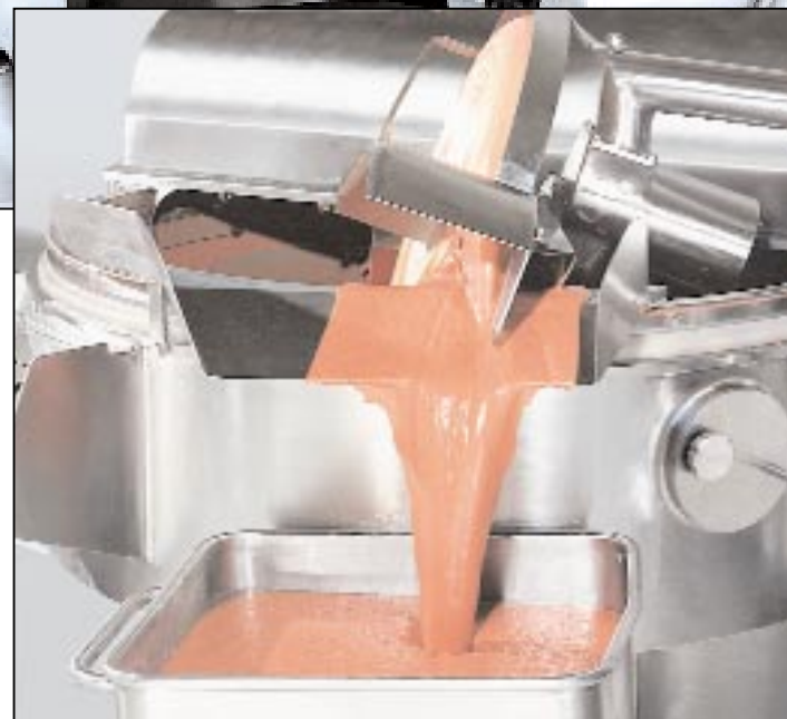
Complete unloading even of liquid material
