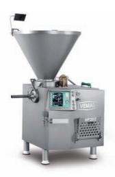
The universal vacuum filler with double screws for flexible use in all applications—the HP20E is the all-rounder among filling machines. Formed, ground or link products and even cold mixtures can be portioned with very little effort, since the VEMAG modular system consisting of vacuum filler and perfectly matched attachments provides maximum flexibility.
