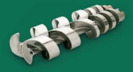
The double screws are at the heart of VEMAG filling machines. The double screws transport even raw materials containing large pieces especially gently all the way from the inlet to the outlet of the machine without a compression zone. The raw material is transported gently and without stress, making your products look ready-to-eat. The double screws operate almost without wearing, reducing
