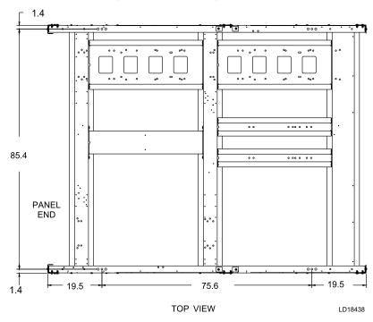
All dimensions are inches unless otherwise specified. Dimensions indicate isolator mounting centerlines.
