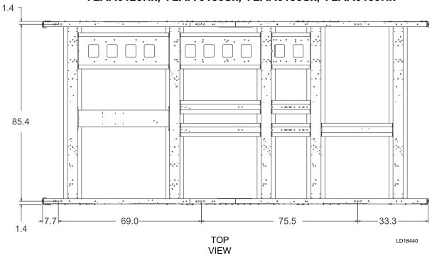
All dimensions are inches unless otherwise specified. Dimensions indicate isolator mounting centerlines.
