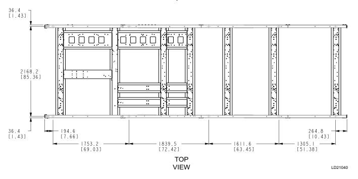
All dimensions are inches unless otherwise specified. Dimensions indicate isolator mounting centerlines.
