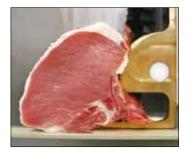
Any product movement can exert a negative impact on the quality of cut. For this reason, the rib stabiliser provides boned goods with extra hold and thus minimises the cutting pressure on the product.
