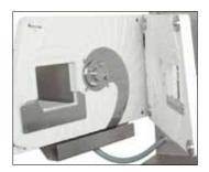
The patented sickle blade is firmly secured between two plates. This so-called sandwich guidance system (stainless steel plates on request) prevents wedge cuts, resulting in clean cuts and increased output.
