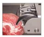
The intelligent gripper recognises which parts of the cutting material are harder (i.e. contain bones) and simply rests gently on these areas. The other hooks hold the meat safely in place.
