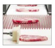
The check weigher and the sorting station are available as optional extras. The tolerance area for deviations from the target weight is set by the operator. Slices which are not of the correct weight are automatically sorted out.
