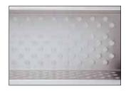
Dimple plate: An air cushion forms between the dimples on which the product is guided to the blade.
