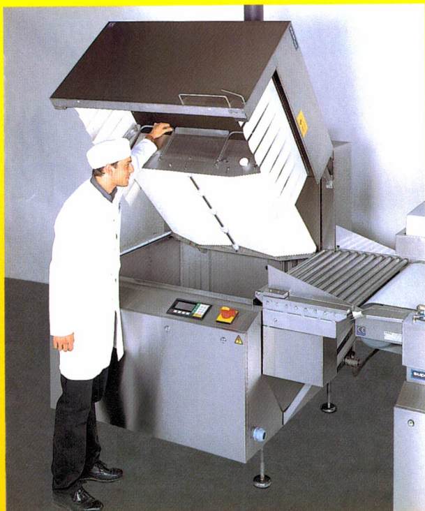
Dipping platform accessible without draining of water. Lid and platform swing upwards and the basin is freely accessible for cleaning.
