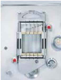
**2** The upper and lower grids are set onto the studs and locked into place by clamps without tools.
