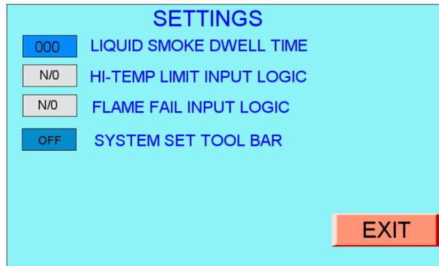
This screen will allow the operator to setup the Liquid Smoke Dwell time default, and Fault Logic.
