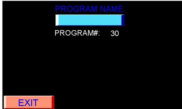
The above screen allows the operator to assign a name and save a program into memory. To save a program, select the Program # you wish to edit and simply set all of the variables in the edit program screen, then click Save Program at the main menu. Name the program appropriately, then push the [EXIT] button. The program is now saved and can be recalled at a later time.
