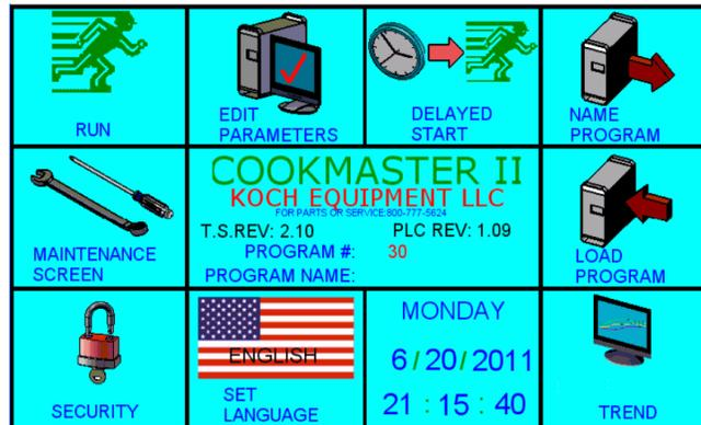
PLC REV: This variable refers to the PLC Software Revision that is currently running.
