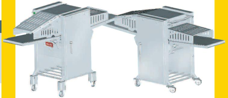
Cubes e.g. from chicken breast can be cut in a second operation or with two machines standing at a 90° angle. The meat passes automatically onto the second machine and needs no second operator.
