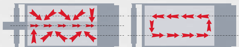
Weiler® twin overlapping, counter-rotating paddle system with unload screw.
